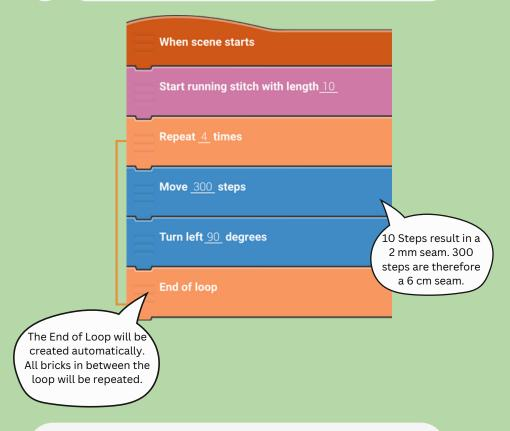
A square is built from four lines, meeting each other in a 90° angle. At first the script runs the running stitch. After that it moves the needle 300 steps and turns 90°. This will be repeated 4 times.
